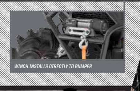
WINCH INSTALLS DIRECTLY TO BUMPER
