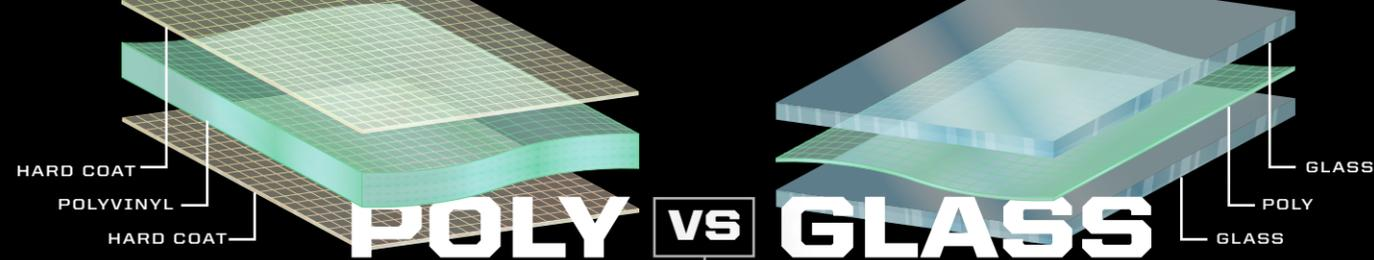
Lightweight and flexible material is **IMPACT-RESISTANT**, providing long-term value and protection. Guarantees a **TIGHT SEAL** to keep out rain and dust. **HARD COAT** provides **30x** more scratch resistance than regular poly.
